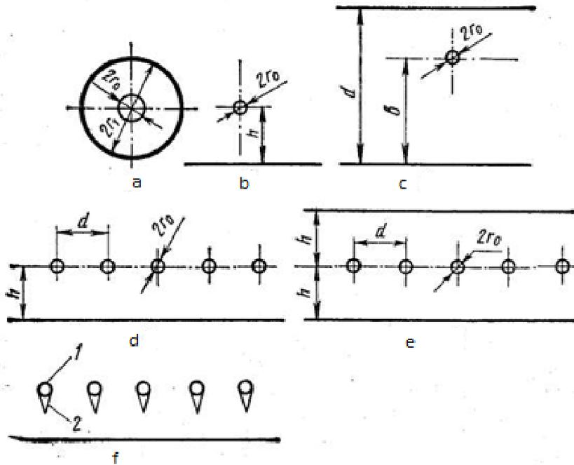
Fig. 1. **Electrode system for creation of the corona discharge field:** a – wire on the cylinder axis; b – wire – plate; c – wire between two plates; d – set of wires-plate; e – set of wires between the plates; f – set of rods with needles – plate; 1 – a rod; 2 – a needle
